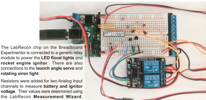
module to power the LED flood lights and rocket engine ignitor. There are also connections to the launch angle servo and rotating siren light. Resistors were added for two Analog Input
